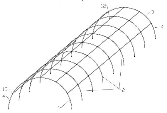
Step D:Install the base rail parts#16,#17 with screws#26 and #28.Bracing with cable#22.
