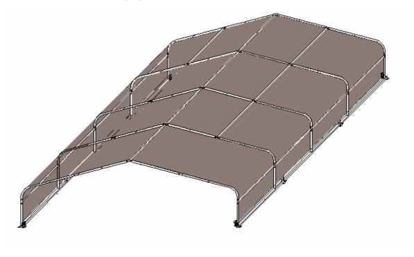
TIPS : Slide the roof cover over assembled frame from one side and insert the conduit to pocket on side:
