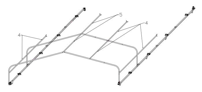
Step C: Install the purlin(4)or(5) as shown below. (use the screws and nuts where necessary)
