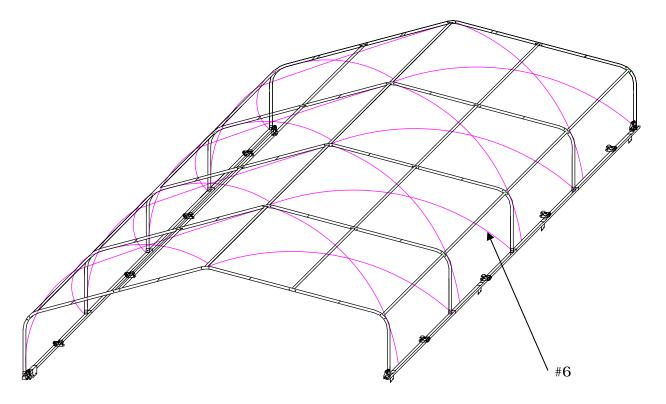
Step E: Put on the roof cover(21) as shown below.
