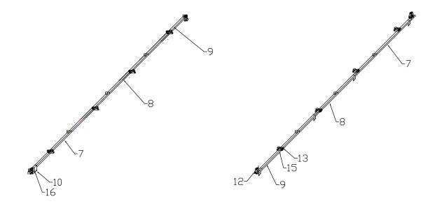
Step A: Place the base rail parts on a chosen place as shown below, and connect the parts.
