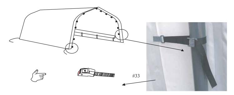
Step2:Attach door cover to frame with Velcro(sewed on cover) band and bungee
